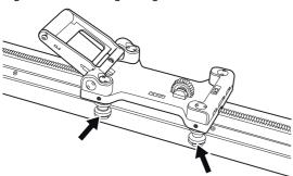
Start by loosening the marked nuts (1) with the supplied special tool. Now loosen the two stop screws (2). When these are loose, adjust the guide wheels (3) against the rail by turning them towards the rail so the play is taken up. Hold the guide wheels and screw in the stop screw. Now screw on the nuts to secure the guide wheels in the new position.
